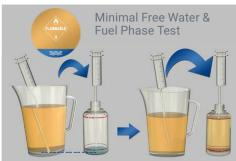
If there is visible free water but not enough to reach the 'Water line' when syringed into the FUELSTAT® test bottle, continue syringing fuel from near the bottom of the sample up to the top line marked 'Fuel line'
