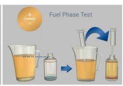
If there is no visible free water in the sample, syringe fuel from near the bottom of the sample into the FUELSTAT® test bottle up to the top line marked 'Fuel line'
