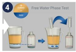
If enough free water in the sample, syringe free water into the FUELSTAT® test bottle to the lower line, marked 'Water line'
