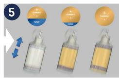
For all types of test, secure dropper cap and shake sample vigorously for 5 seconds
