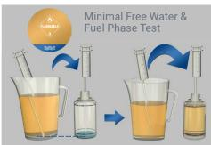
If there is visible free water but not enough to reach the 'Water line' when syringed into the FUELSTAT® test bottle, continue syringing fuel from near the bottom of the sample up to the top line marked 'Fuel line'
