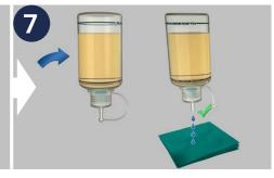
Fully invert the bottle and allow 4 drops to spill onto a tissue to clear the dropper nozzle of any trapped fuel deposits, **DO**
