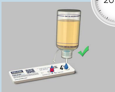
put 4 drops into test well
