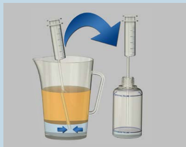
once settled, extract into test bottle
