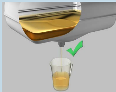
collect fuel sample from fuel tank
