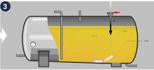
Lower the Aquafighter into the tank low point location so that the Aquafighter is resting on the bottom being lightly suspended in the tank, using the mark on the cord as reference
