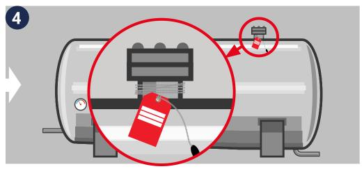
Ensure that sufficient length of cord is left outside the tank so that it can be attached, e.g. by making a loop around the exterior of tank filler pipe opening, or other suitable secure attachment
