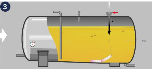
Lower the Aquafighter into the tank low point location so that the Aquafighter is resting on the bottom being lightly suspended in the tank, using the mark on the cord as reference
