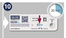
Leave the FUELSTAT° test cassette on a flat surface for **15-20 minutes**. A dark red line 'Control line' should appear on the left-hand side of the viewing window. This indicates that the test has worked correctly
