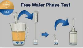
If there is free water in the sample, use the supplied **20ml syringe and tube** to extract **free water** from the bottom of the sample and place into the plastic cup Then use the supplied small **1.0ml syringe** to extract just **1.0ml** of **free water** from the plastic sample cup and place into the FUELSTAT® test bottle
