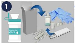
Clean sample equipment using 70% alcohol wipes and let dry. Have the FUELSTAT<sup>®</sup> One test kit contents at hand. Wear correct PPE, including Nitrile gloves and safety eyewear when handling fuel
