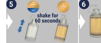
For both types of test, secure dropper cap onto the bottle with the sample and **shake sample vigorously for 60 seconds**
