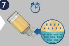
Gently invert test bottle 45° and allow the blue fluid to settle out in the shoulder of the bottle.
