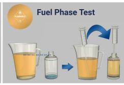
If there is no free water in the sample, use the supplied **20ml syringe and tube** to extract **fuel** from near the bottom of the sample and place into the FUELSTAT<sup>®</sup> test bottle. Repeat until filled up to the line marked '**Fuel line**'
