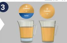
Agitate sample using a swirling motion and leave to **settle for 12-15 mins**. Once settled, is there any free water at the bottom of the sample?
