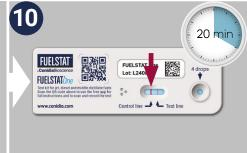
Leave the FUELSTAT° test cassette on a flat surface for **15-20 minutes**. A dark red line 'Control line' should appear on the left-hand side of the viewing window. This indicates that the test has worked correctly
