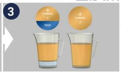
Agitate sample using a swirling motion and leave to **settle for 12-15 mins**. Once settled, is there any free water at the bottom of the sample?
