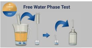
If there is free water in the sample, use the supplied **20ml syringe and tube** to extract **free water** from the bottom of the sample and place into the plastic cup
