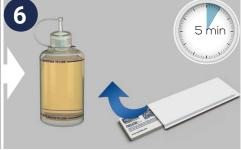
For a fuel sample test leave the FUELSTAT® test bottle contents to **settle for 5 mins**. In the meantime remove the FUELSTAT® One test cassette from the sealed foil packet and place on a clean flat surface
