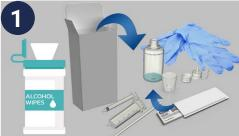
Clean sample equipment using 70% alcohol wipes and let dry. Have the FUELSTAT® One test kit contents at hand. Wear correct PPE, including Nitrile gloves and safety eyewear when handling fuel
