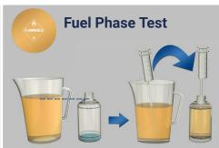
If there is no free water in the sample, use the supplied **20ml syringe and tube** to extract **fuel** from near the bottom of the sample and place into the FUELSTAT® test bottle. Repeat until filled up to the line marked '**Fuel line**'
