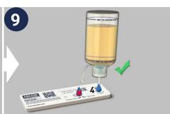
Keep the bottle inverted and carefully allow 4 drops of blue fluid to fall into the circular well on the test cassette as indicated ensuring that no sample is spilled into the viewing window
