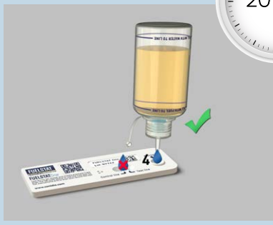
put 4 drops into test well
