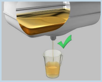
collect fuel sample from fuel tank
