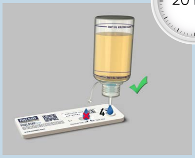
put 4 drops into test well
