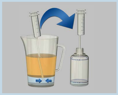
once settled, extract into test bottle
